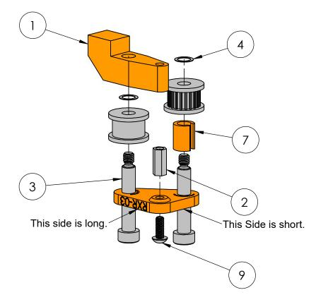
Note the orientation of the Reinforcement Plate
