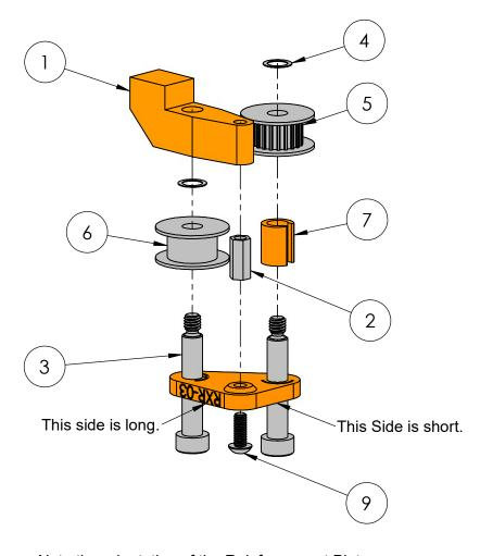
Note the orientation of the Reinforcement Plate
