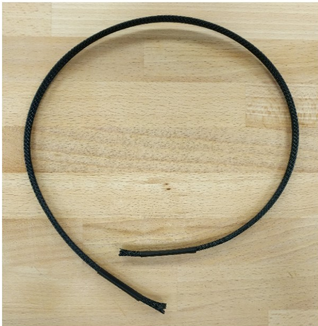
Cut 750mm of 1/2-in. cable sleeving. Slide two 10mm bits of heat shrink tubing onto the ends.
