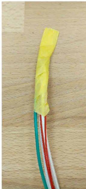
Collect the thermistor wires, grounding wire, and bed heater wires into once bunch. Tape the far ends together and run the bunch all the way through the cable sleeve.
