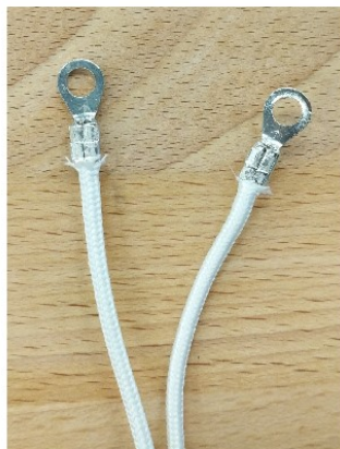
Crimp Ring terminals on the bed heater wires. From the Duet Ethernet box, crimp two small pins from the loose bag and click them into a two-prong connector.
