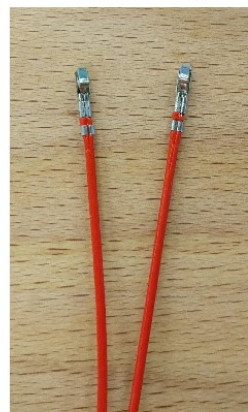
Crimp Ring terminals on the bed heater wires. From the Duet Ethernet box, crimp two small pins from the loose bag and click them into a two-prong connector.
